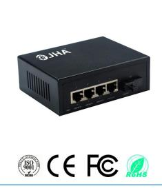
JHA-F14 series is complies with IEEE802.3 standards, It is designed to convert data signal between 100Base-FX and 10/100Base-T(X) fast Ethernet.
